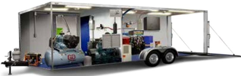
we custom-build trailers to meet your specifications. ArmorThane has all of the high-pressure and low-pressure equipment and supplies needed to be fast and efficient.
